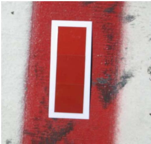
**FIGURE 6-72. RED COLOR CHIP COMPARED TO RED MARKING.**
