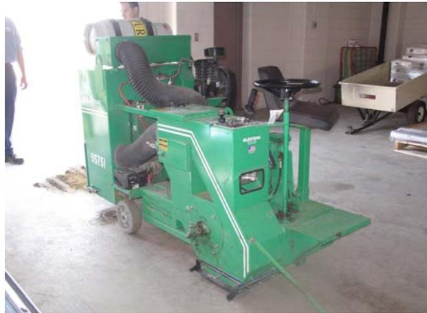
**FIGURE 5-13. SHOTBLASTER WITH A 10-INCH CUT.**
