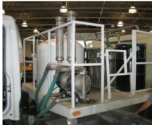
**FIGURE 6-29. PNEUMATIC TRUCK-MOUNTED SYSTEM.**
