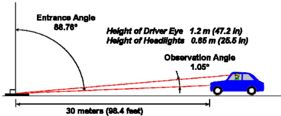
**FIGURE 3-1. 30-METER GEOMETRY**
