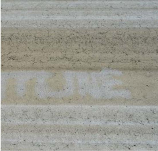
**FIGURE 4-30. RUST REMOVER WHITENS STAINED MARKING WHERE “TLINE” WAS PRINTED.**
