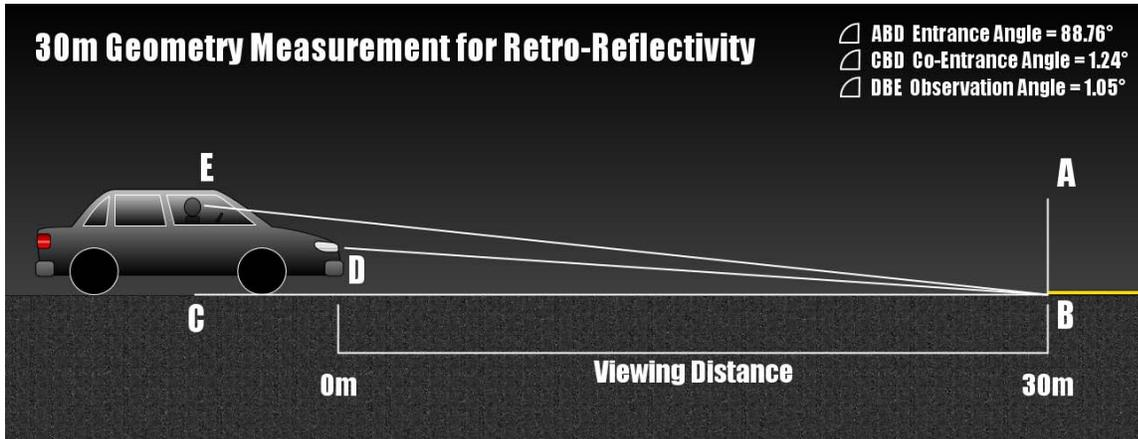
**FIGURE 1 - Thirty-meter geometry measurement for retro-reflectivity evaluation.**
