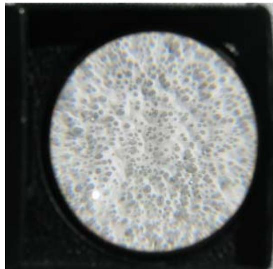
**FIGURE 3-5. GOOD TYPE I BEAD DISTRIBUTION; READINGS AVERAGED 300 mcd/m<sup>2</sup>/lux.**
