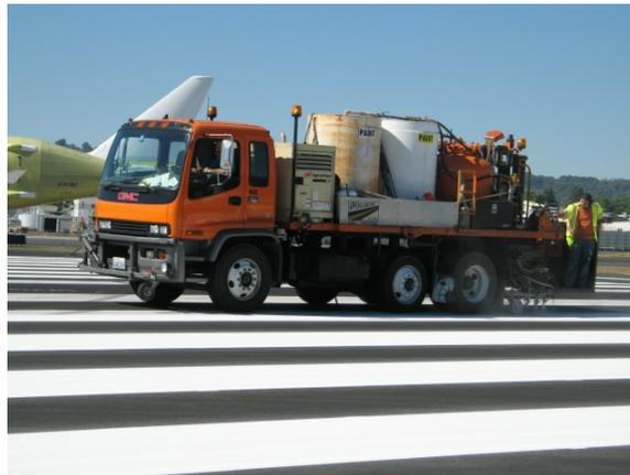
**FIGURE 6-25. TRUCK MOUNTED STRIPING EQUIPMENT WITH LARGE MATERIAL TANKS.**
