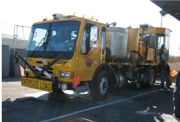
**FIGURE 6-24. TRUCK-MOUNTED AIRPORT STRIPING EQUIPMENT.**
