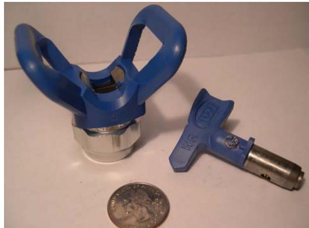
**FIGURE 6-19. AIRLESS FAN WITH TIP.**
